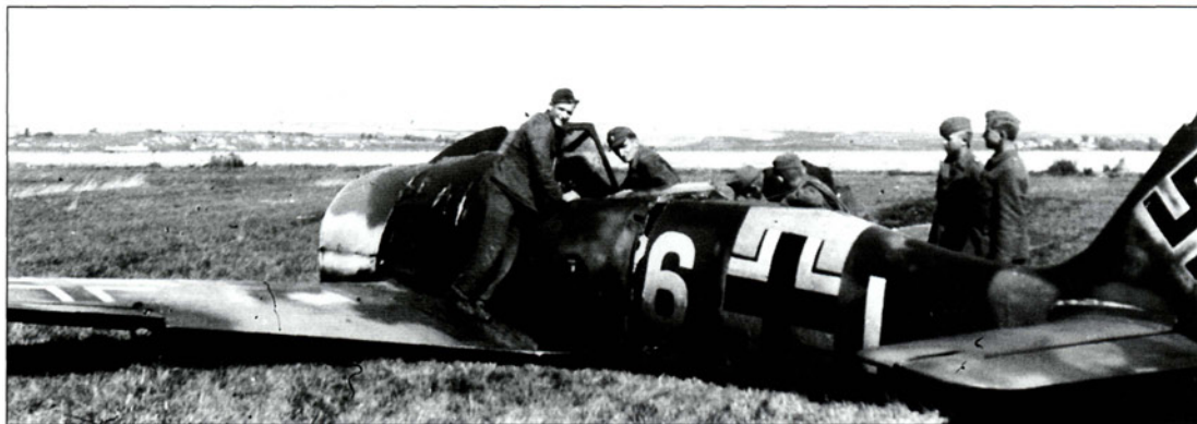
Aircraft losses were mounting too. Although the unknown pilot no doubt survived this neatly executed belly-landing near Czemlysh in August, 7. Staffel 's 'White 6' has split open aft of the cockpit and now lies broken-backed – a total write-off
